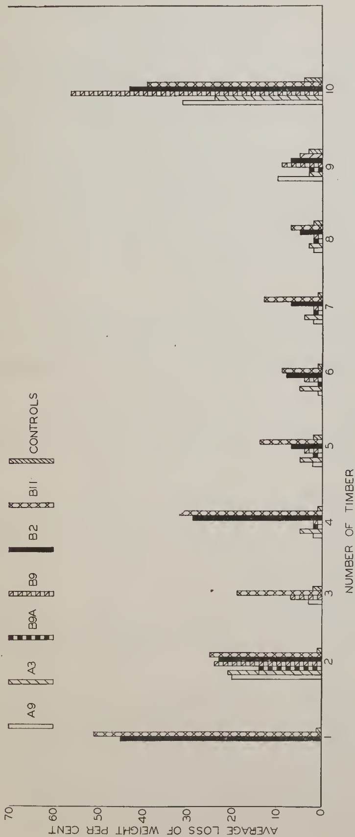
GRAPH 3. EFFECT OF VARIOUS FUNGI ON TEST TIMBERS AT 30 PER CENT MOISTURE CONTENT OF SOIL
